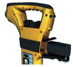
The battery can be charged in situ. Unscrew the ½ turn fastener of the battery compartment (do not open the internal battery door). Align the red dot on the charger plug with the dot on the charging socket and connect together. Connect the supplied charger to the mains and switch on. The charging LED on the charger will illuminate red until the batteries are charged. The LED will then turn green indicating a full charge.
