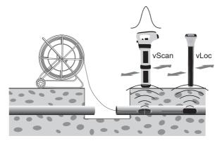
Finally check the locator is in line with the sonde by rotating it on its axis to obtain a peak signal. The Vscan is now over the sonde and in line with it. For the vLoc this indicates the sonde being across the line of the sonde. Note that it should not be necessary to adjust the gain again unless the depth of the pipe changes significantly.
