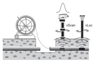
If a depth estimation is required. Place the locator on the ground having pinpointed the sonde as above. Momentarily press the "I" button and the depth will be displayed. To exit the depth screen, either wait for the depth screen to "time out" or momentarily press the on/off key which will return the vScan to the locate screen. (For the vLoc press the "I" button to exit the depth screen)
